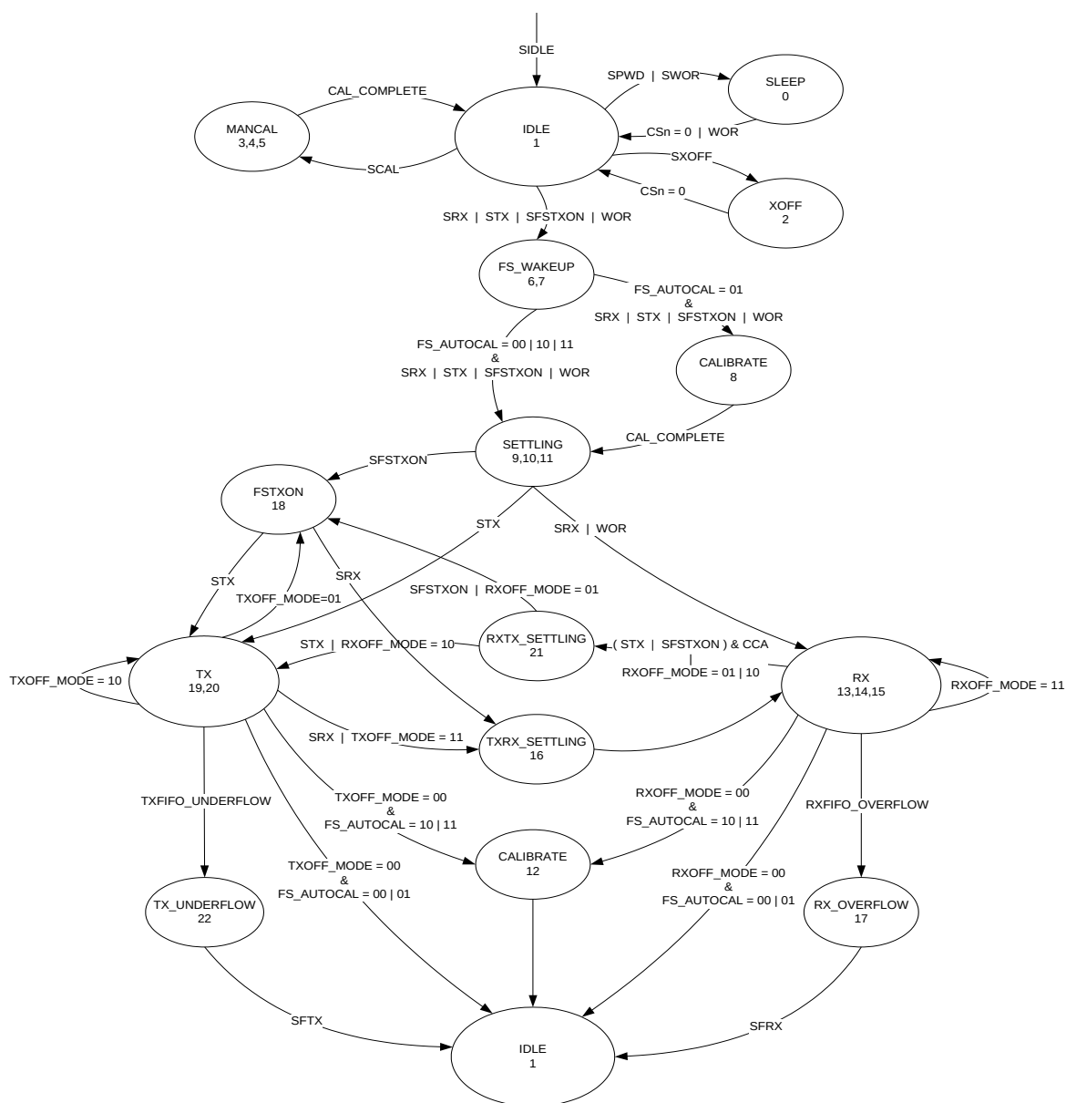
Figure 25: Complete Radio Control State Diagram
